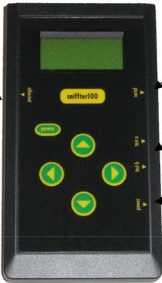
The Sniffer displays information on a 20-character wide, 4-line, backlit LCD display. Press and release the power button to turn the Sniffer on. To turn the backlight on or off, hold the power button down for 3 seconds (until the backlight changes) and then release.
