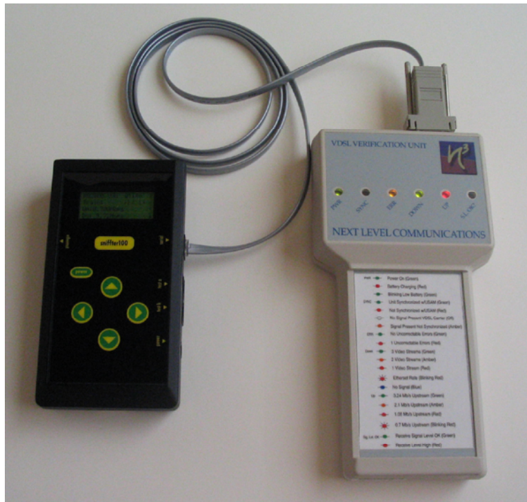
VVU connected to Sniffter serial port with male serial adapter and regular (straight through) RJ12 phone cable.
